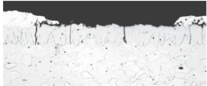
Coating Pit on 30-year old pipe demonstrating arrested pit penetration.
